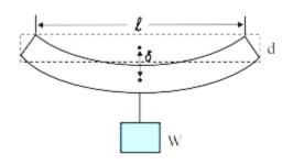
A bar of length I, breadth b, and depth d when loaded at the centre by a load W sags by an amount given by  $\delta = W I^3/(4bd^3Y)$
